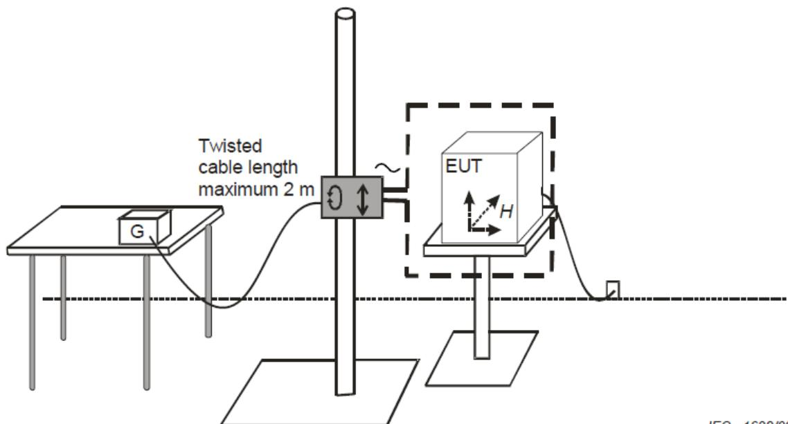
Test set-up for floor-standing equipment
